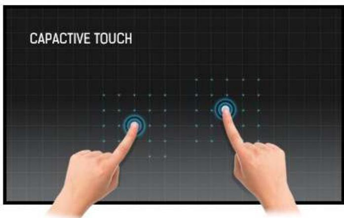
This technology uses a sensor-grid of micro-fine wires integrated into the glass that covers the screen. Touch is detected because electrical characteristics of the sensor grid change when human finger is placed on the glass. Thanks to the glass overlay this technology is highly durable, and the touch function remains unaffected even if the glass is scratched.
